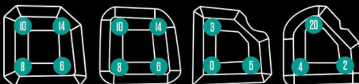
*The numbers represent the size (in millimetres) of the finished silicone bead, whether it is square, round, or flat.*
