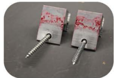
No Water Penetration
